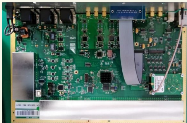
Figure 2: Assembled UUB unit, equipped with front panel, GPS receiver, cables, and shielding covers.
